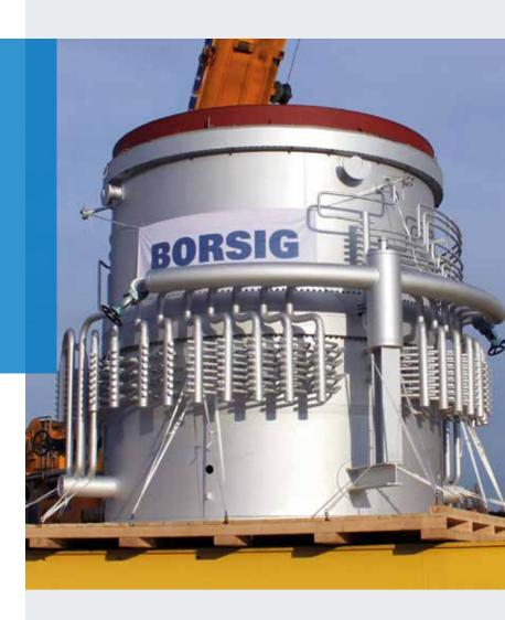
Process gas coolers/waste heat boilers with direct integrated reactors are used in the production of nitric acid, caprolactam and formaldehyde.
