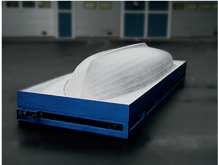
Fig. 4. An approx. 2500kg, high-quality thermoforming boat-mold that can be molded perfectly, even at the edges © Alwa
