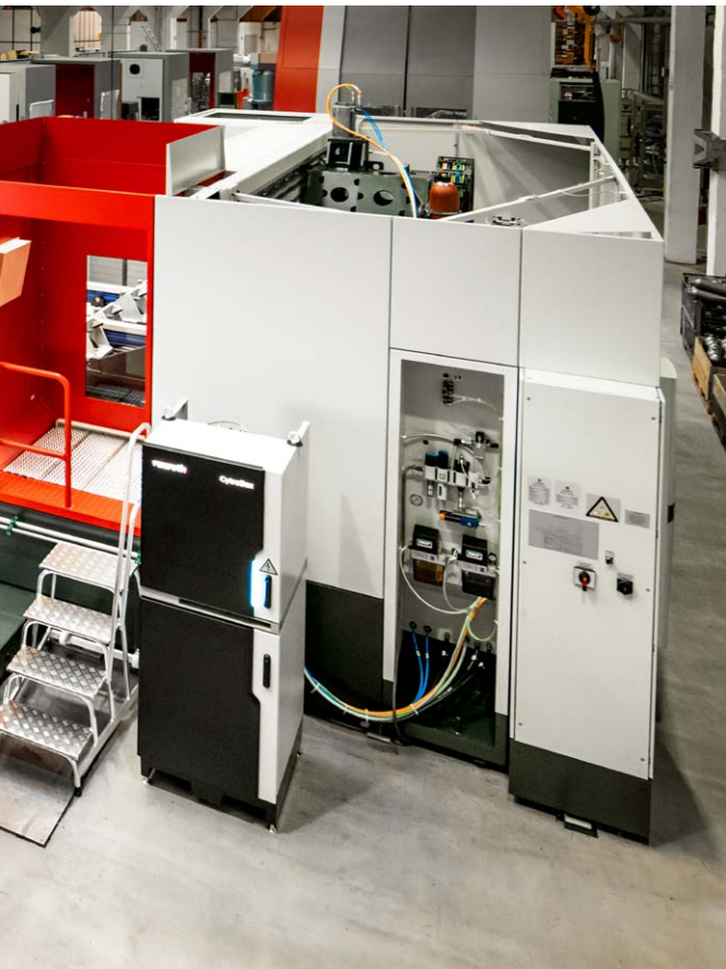
Association of two SFZ 2500 to form a special machine
