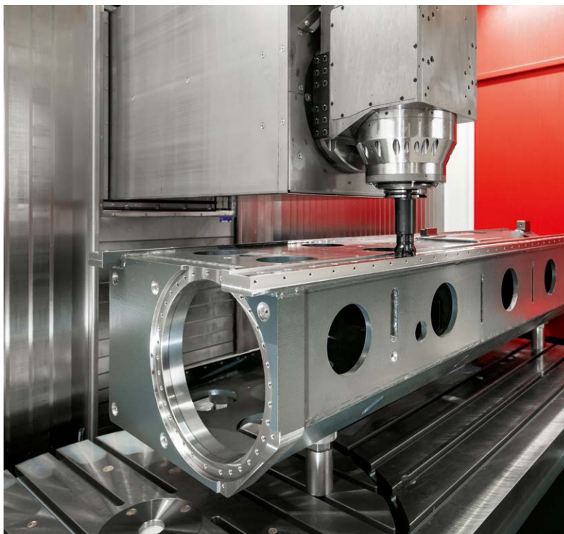
Vertical machining of the guideways of a Y-slide
