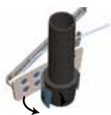
2. Positioning of the label around the mandrel
