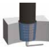
3. Inserting the label into the mould
