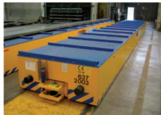
Machines designed to be able to transport sheet coils and other heavy materials along a transversal path with respect to the adjacent industrial buildings.
