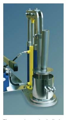
The pressing units built by PC Laborsystem can be delivered as manual operated or hydraulic operated systems. They are designed for a pressure of up to 15 bar on the product, are suited for middle to high viscous products and vessel sizes of up to 400 mm in diameter.
