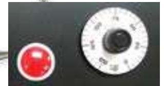
Easy-to-set dial controller within NEMA 4X enclosure
