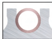
Kupfer-Nickel-Kühlkanal* copper-nickel cooling channel*
