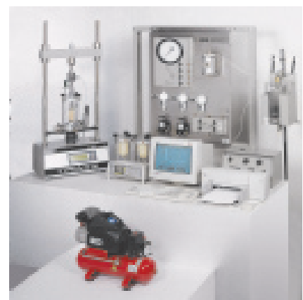
Typical configuration of an advanced single cell triaxial testing system with electronic measurement and data acquisition and processing. Bladder type air/water pressure system.
