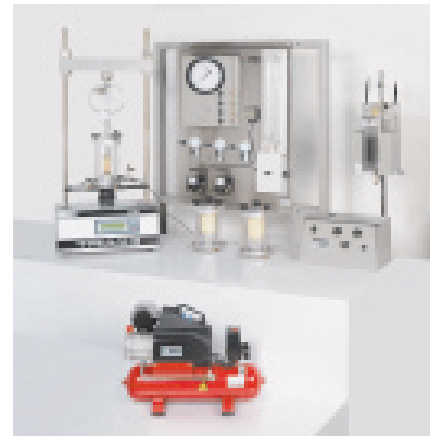
Typical configuration of a testing set for the determination of the consolidated undrained (CU) and consolidated drained (CD) triaxial test with measurement of pore pressure and volume change. Bladder type air/water pressure system and de-airing water system.
