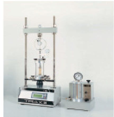
Typical configuration of a basic standard testing set for the determination of the undrained shear strength (total stress - UU) in triaxial compression on Ø 38 mm specimens. Oil and water pressure system
