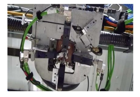
Four Laser Scanners with blue laser lines scan the position of the gluebead in 360° position as well as the width and height
