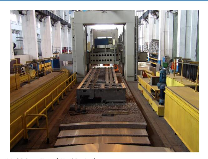
Machining a Casted Machine Bed
