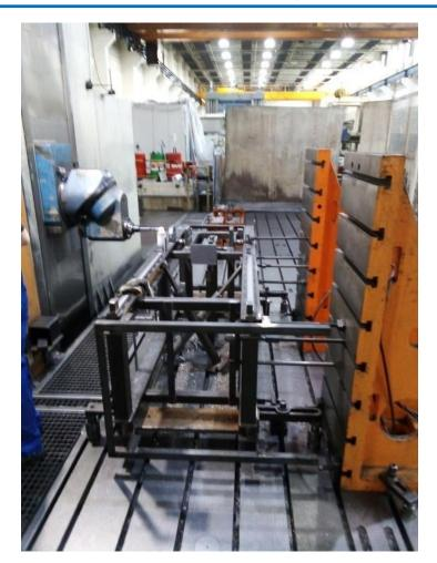
Machining a Steel Structure
