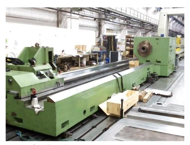
Reworking of a Roller Lathe
