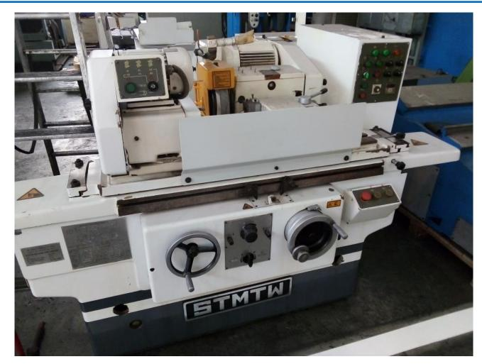
• Smaller Cylindrical- Grinding-Machine STMTW MMB1420 C
