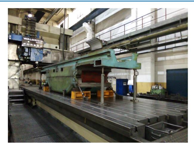
Removing of old worn-out guideways by milling
