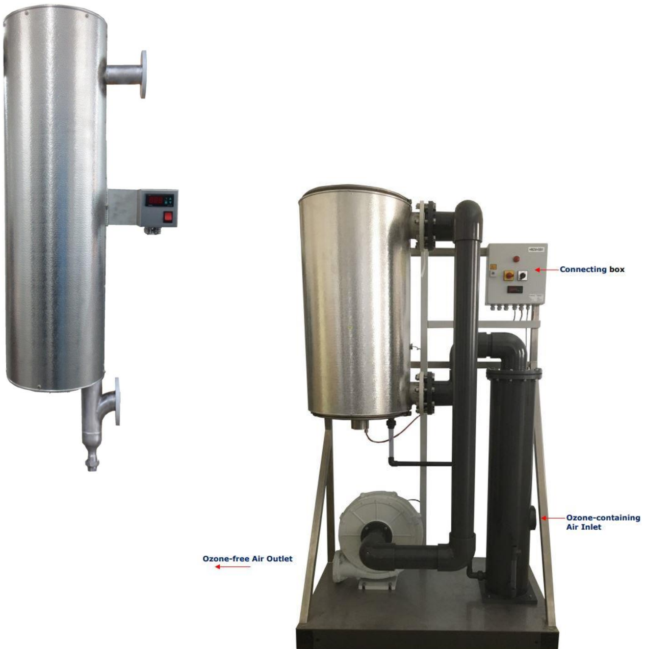
Skid assembly with suction fan and foam separator
