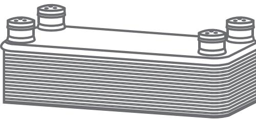
The maximum working pressure is 30 bar. The working temperature is included between -160° and +225°C. The maximum difference between the temperatures of the fluids is 100°C. For each type of exchanger, the thermic performance's curves, as a function of the oil rate, show the heat quantity in kW or in kcal/h that the exchanger is able to dissipate for each degree of difference between the inlet temperatures of water and oil.
