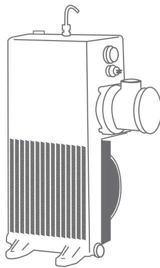
This is a special type of heat exchanger with incorporated tank and filter. It is suitable for the cooling of hydrostatics transmissions in off-line circuits, above all on concrete mixers, and allows simplifying the hydraulic system and reducing in this way its cost.
