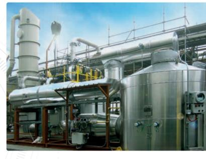
A catalyst is used to reduce the reaction temperature and therefore the energy consumption. This allows the oxidation process to be performed at lower temperatures between 300°C and 500°C, which leads to considerable energy and cost savings.
