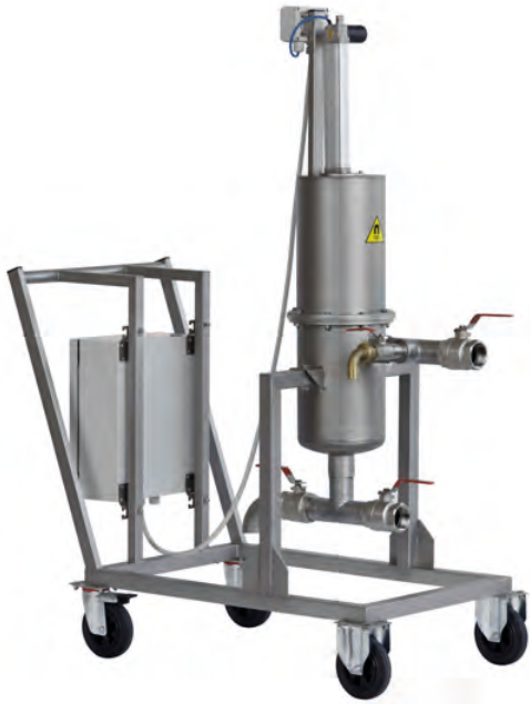
FDA (9000 lt/hr - 13500 Gauss) Filtro deferrizzatore autopulente Auto-cleaning iron remover filter
