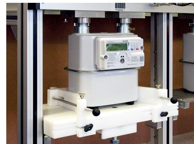
meters as well as for industrial gas meters. The constructive design of the devices enables clamping of a large number of different meter sizes and meter connections. This contains additional meter components as there are inlet sections or outlet sections or flow straighteners. The delivery range contains as well the upgrading of existing inotech test rigs or other brand test rigs.
